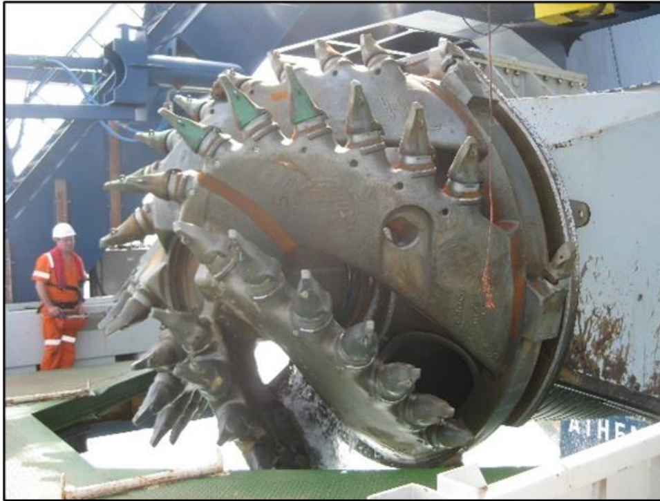
Figure 2: Cutterhead of the Athena CSD
